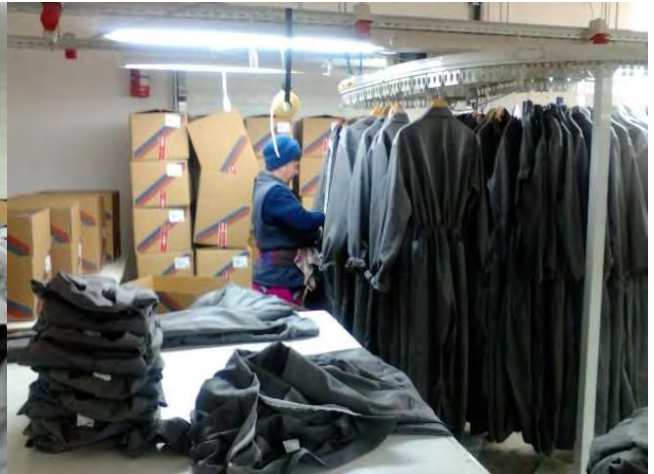
Photo caption: Workspace to clean the finished product and conduct final controls for packaging, equipped with a hanging conveyor after MCP assistance.
