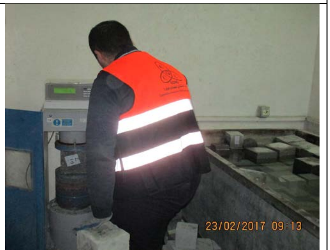
Photo No.04.2: 28 Days` compressive strength test of CEM II 1 st trial mix concrete cubes at CCQC Lab in Gaza. Date: February 23, 2017
