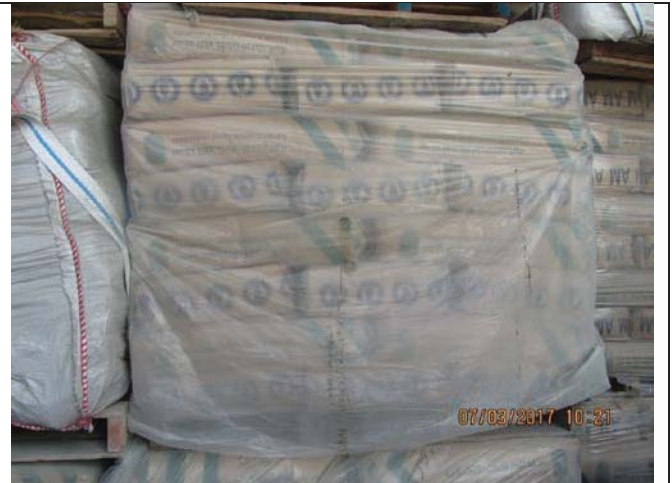
Photo No.02: Cement CEM II (source: Nesher, supplier: SANAD).
