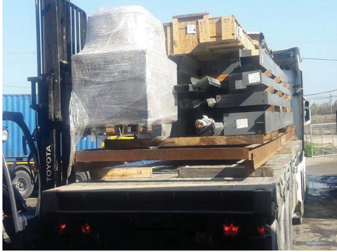
Photo No.45: Delivery of Pre-engineered steel structures. Date: January 30, 2018
