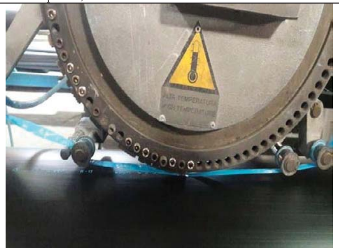
Photo No.22: Site visit to Plassim Factory (Israel)-Marking on pipes and fittings.
