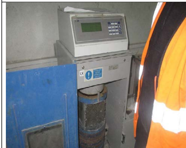
Photo No.03.2: 7 days compressive strength test of CEM II concrete cubes at the CCQC Lab-Gaza Strip. Date: February 02, 2017
