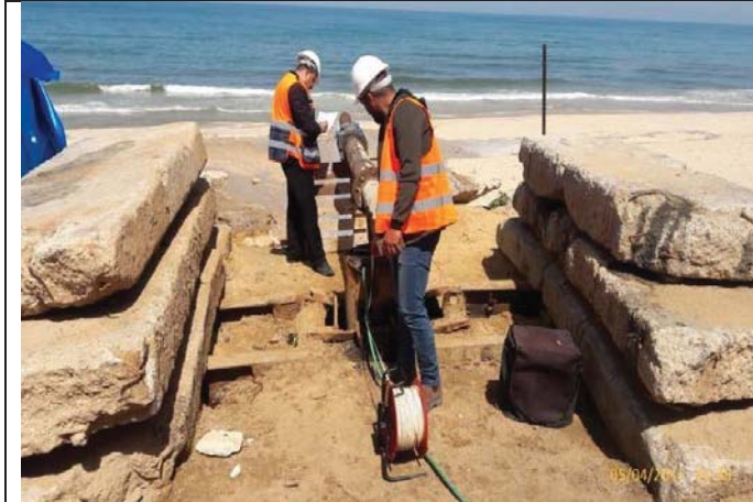
Photo No.05: Continue hydrogeology investigation for beach wells borehole (pumping test). Date: April 05, 2017
