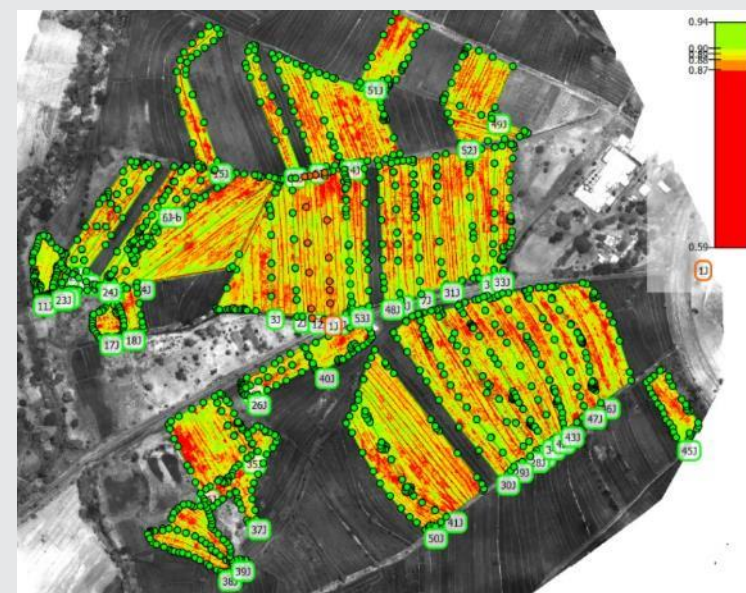
The boundaries of farmers' fields were mapped using drone-mounted GPS in a fraction of the time required if undertaken by walking.
