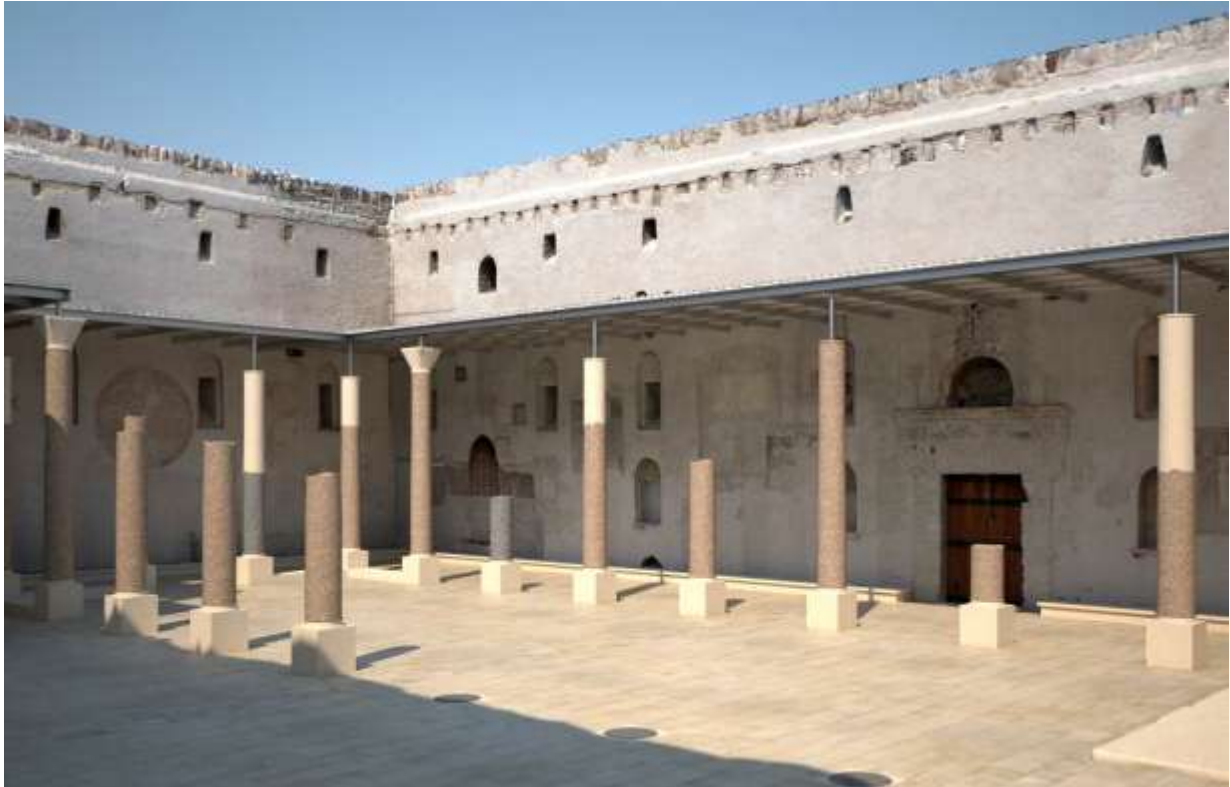
Figure 9: Computer model of the nave showing proposed location of protective shelter and extent of shade on 25 March 2019 (image: P. Gasparri. 2019)
