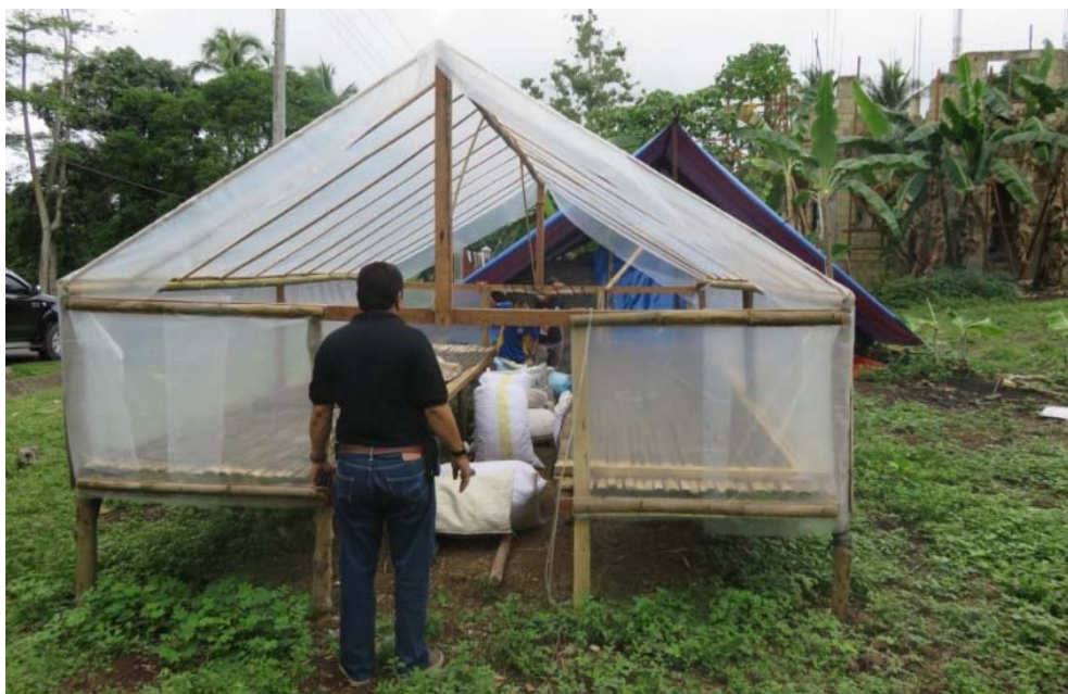
The papag dryer which has a UV plastic roofing and enclosure enables the association to dry cassava chips even during inclement weather. It protects the chips from contaminants such as soil and dust that affect over-all product quality.
