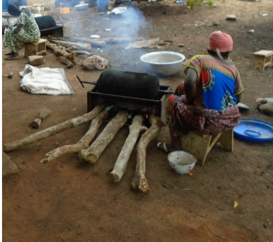
Figure 3. Roasting drum in Wechiau - Roasting time is ~50minutes
