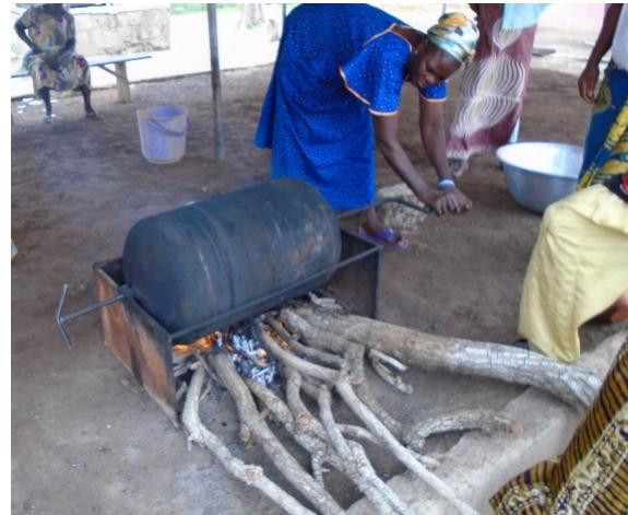
Figure 4. Roasting drum in Tamale - Roasting time is longer than 1 hour
