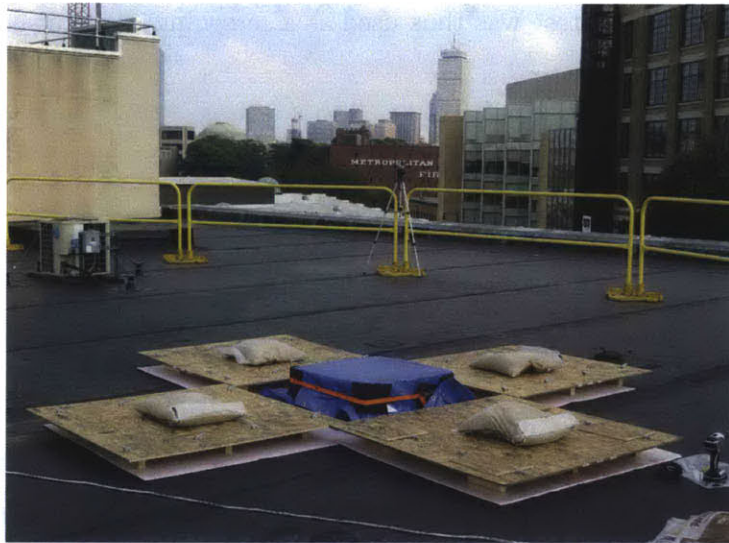
Figure A-2: Solar lantern charging station. This charging station is located on the roof of building N51 at MIT. Solar lanterns were placed on these platforms for the charging tests.
