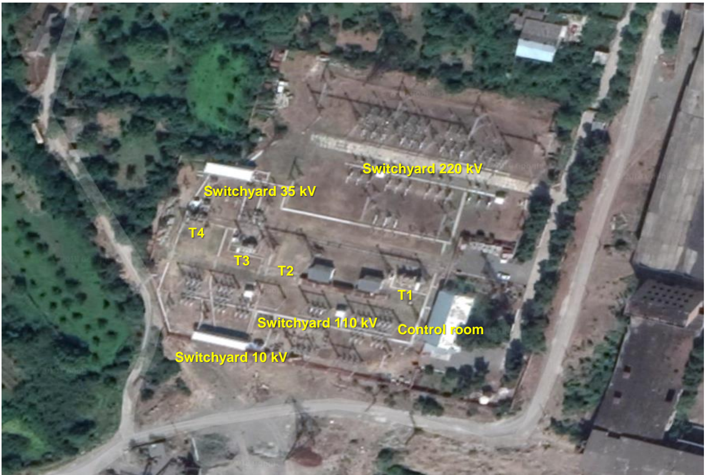
Fig 3. Map of Substation Gori
