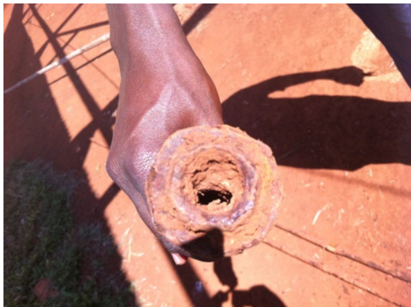
Figure 4.5 Encrustation of the ½ inch pipe removed from the CBD during a leak repair exercise
