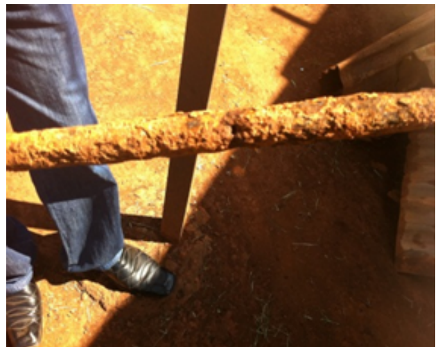
Figure 4.5 Encrustation of the ½ inch pipe removed from the CBD during a leak repair exercise
