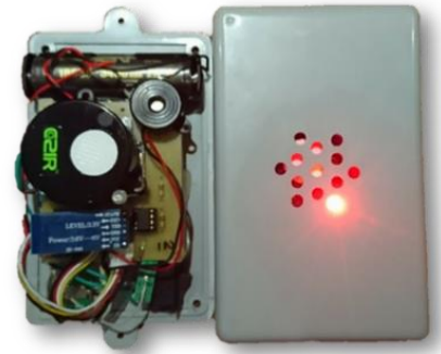
Figure 16: A CO 2 monitor developed by the project
