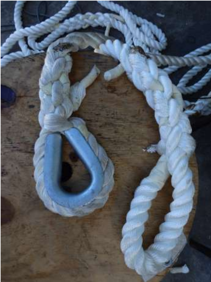
Figure 27. Image of a pickup line made with a spliced rope loop reinforced with steel (Reed, 2016).
