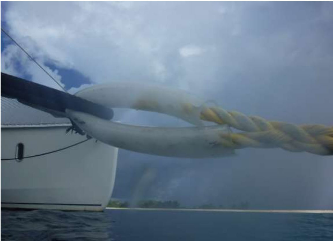
Figure 23. Image of the standard pick-up line with spliced rope loop reinforced with plastic piping to reduce abrasion from vessel lines (Reed, 2016).
