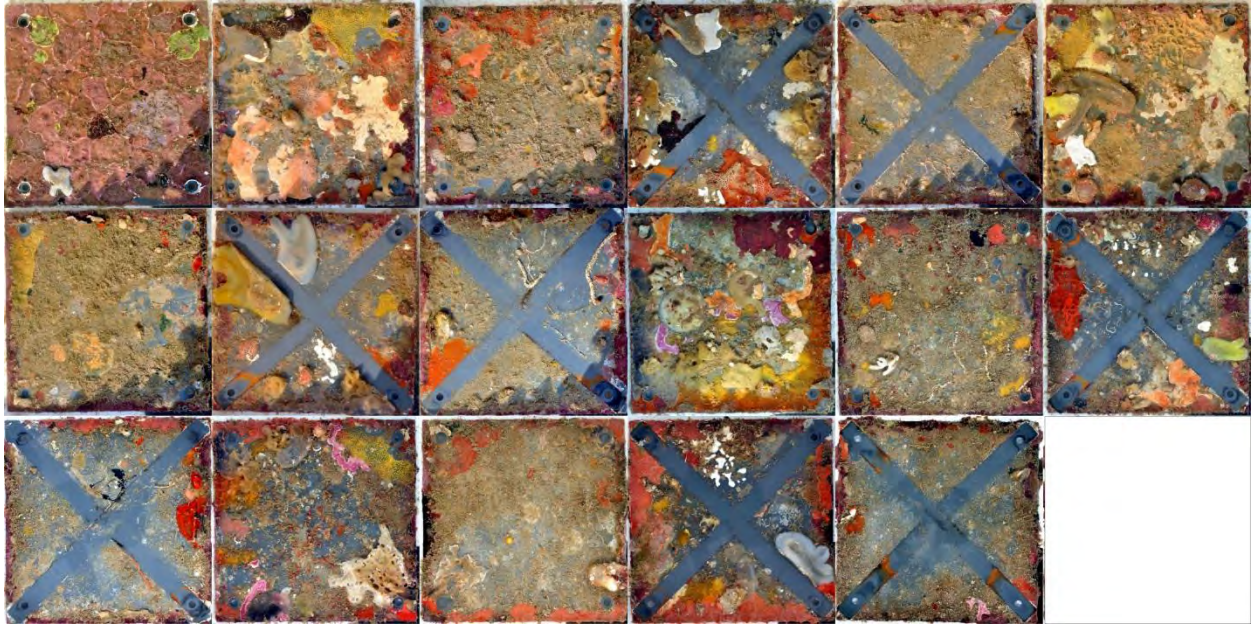
Figure 69. Photos of the ARMS plates from an ARMS unit recovered from site BOB-02. There are 9 plates per ARMS unit, with the topside and underside of each plate photographed except for the bottom plate that had only the topside photographed since the underside was resting on the base plate, for a total of 17 photos per ARMS unit. ARMS plate photos are displayed starting from the top plate in the upper left corner moving in a left to right direction for each row of photos. The photos with the cross hatches represent semi-closed layers.
