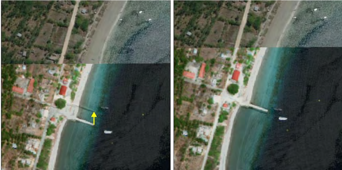
Figure 59. Side by side figures showing a WorldView-2 satellite image overlaid on top of the reference basemap before ( left ) and after ( right ) georeferencing. Partial transparency is applied to the WorldView-2 image, thus features in the reference basemap in the background are visible through the WorldView-2 image in the foreground. The positional error is apparent when comparing the location of a structure between the WorldView-2 satellite image and the reference basemap (yellow arrow).
