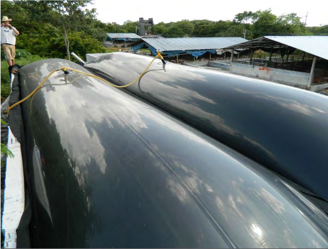
Image 4: 80 cubic meter tubular modular polyethylene biodigester at a medium scale hog farm in Yucatan (2013).
