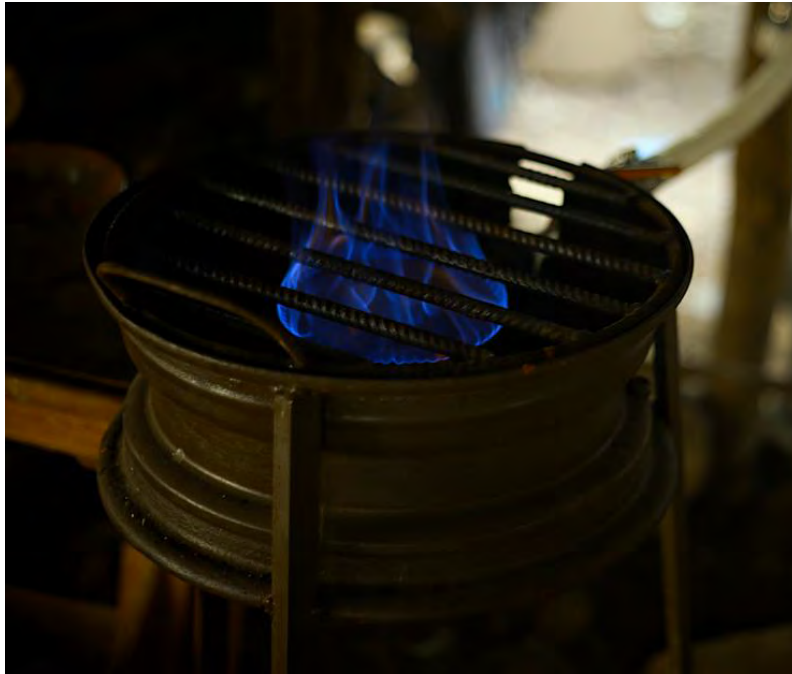
Image 8: The indicative blue flame of methane combustion in domestic biodigester application in Yucatan
