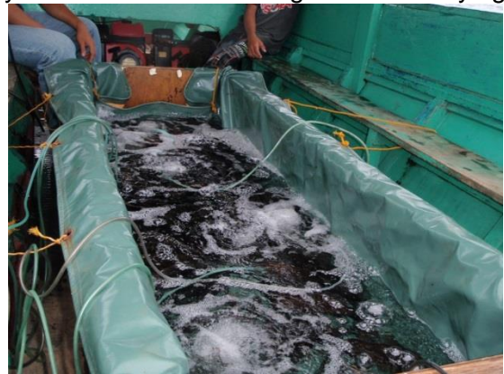
Live fish transport system installed on boat
