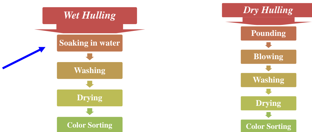
Figure 3: Process involved in Wet & Dry Hulling
