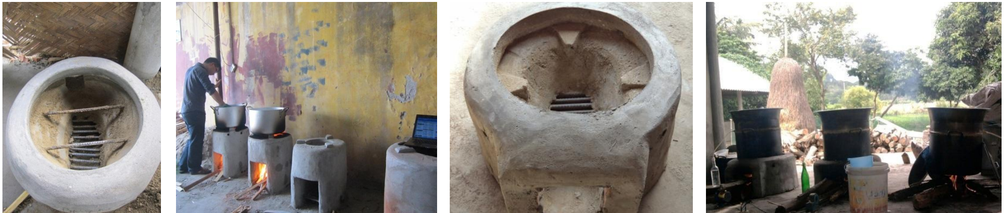
PICTURE 8: FROM LEFT TO RIGHT: DK-TK PILOT STOVE BUILT IN THE FIELD: WATER BOILING TEST IN HANOI: DK-TK 06, PROVEN PERFORMANCE IN THE LAB BUT NOT IN THE FIELD; CONTROLLED COOKING TEST IN THE TARGET AREA
