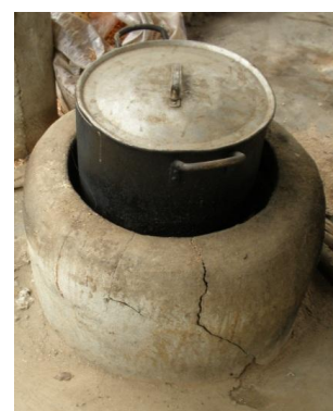
FIGURE 19: A CRACKED STOVE IN THE TARGET AREA
