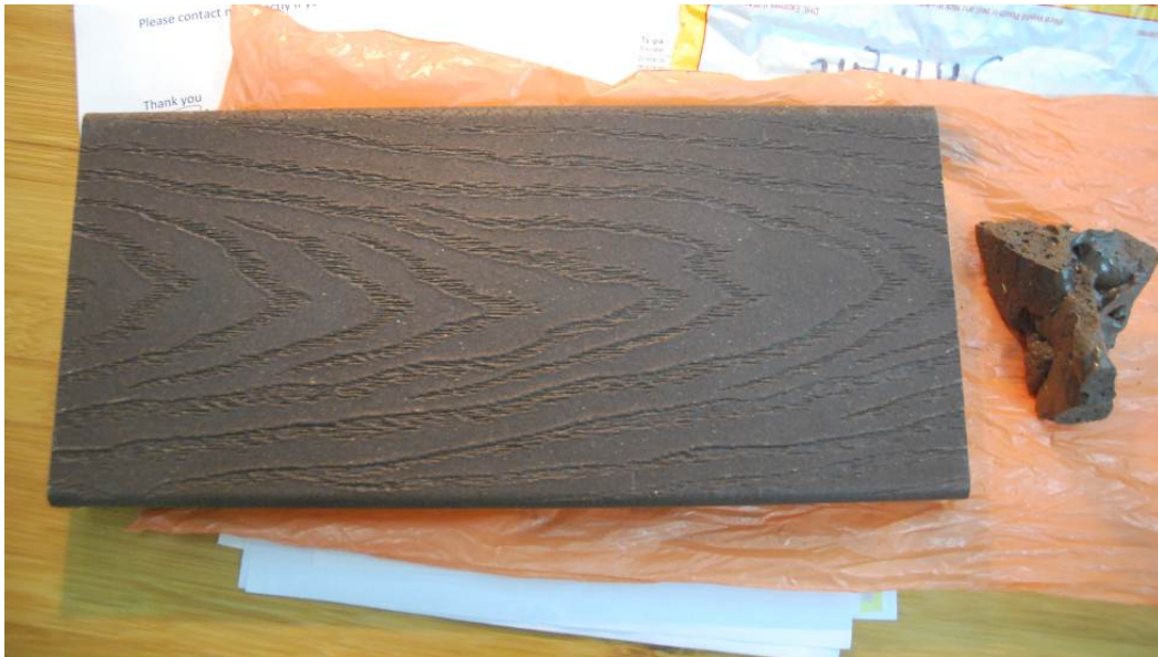
On the left: bio-composite plastic wood board created out of recycled PE LLINs by Trex. On the right: recycled PET nets unable to be manufactured into a board.
