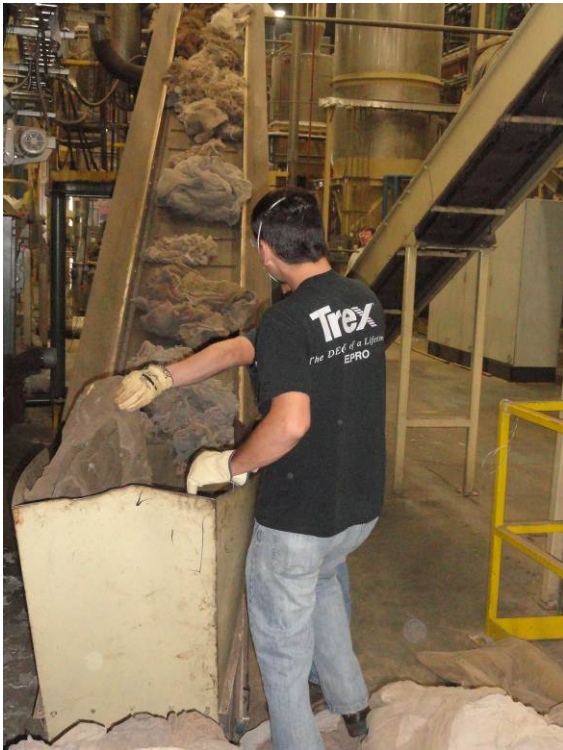
Trex staff members load nets onto the densifier
