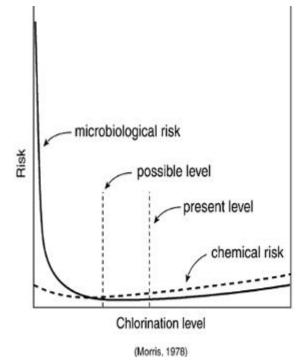
Figure 1– The Inverse Relation between Risk and Chlorination Level. Note how chemical risk tends to stay constant over chlorination level deviations.
