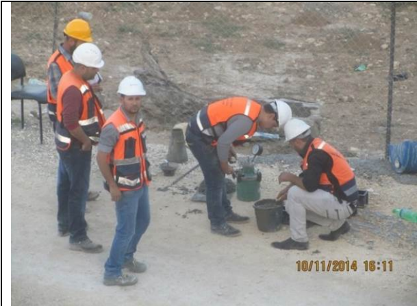
Arraba Well: Collecting concrete samples and field tests for balance tank walls (section E2)
