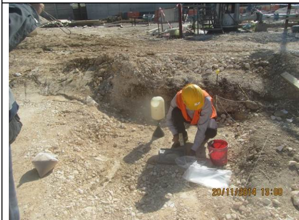
Sanur Well: Collecting of compacted base course samples under chlorination room foundation
