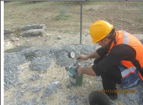
Arraba Well: Collecting concrete samples and field tests for balance tank walls (section E1)
