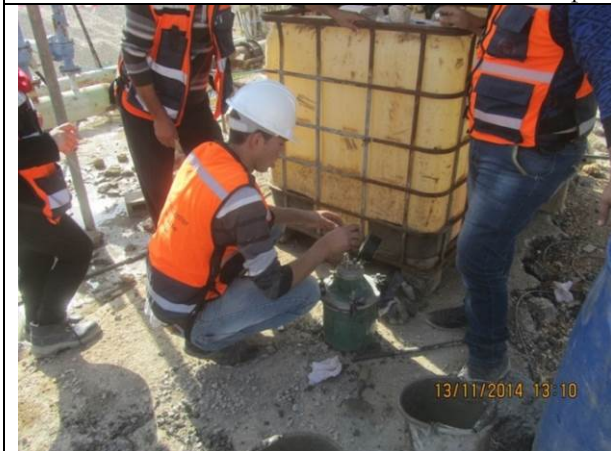
Sanur Well: Collecting concrete samples and field tests for balance tank walls (Section E1) and fence wall foundation segment AB.
