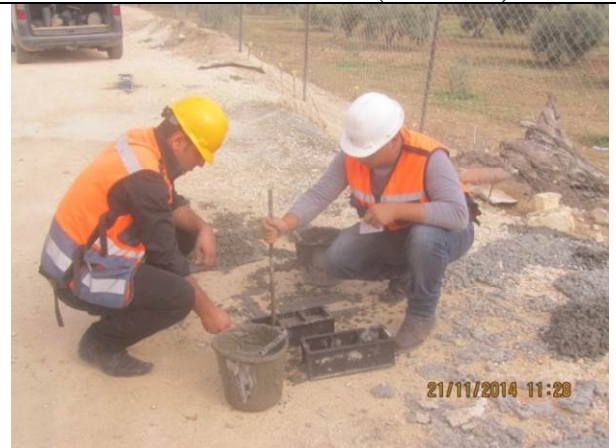
Arraba Well: Collecting concrete samples and field tests for balance tank walls (section E1)
