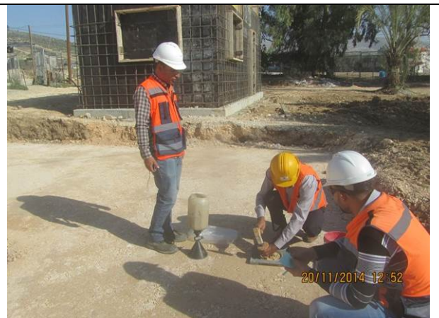
Sanur Well: Collecting of compacted base course samples under chlorination room foundation
