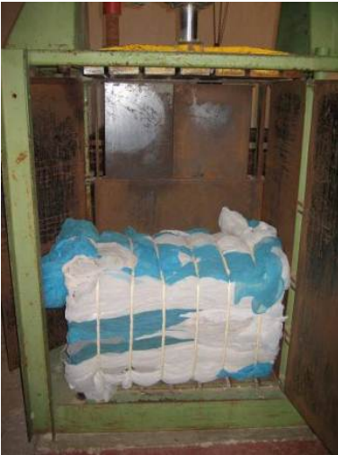
Sisal press used to compact LLINs.
