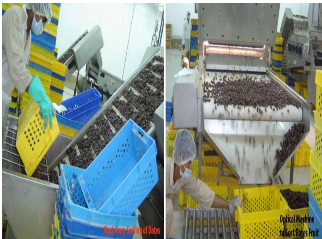
Figure 46: Machinery Sorting of Dates According to their Sizes in Al-Saad Factory, UAE
