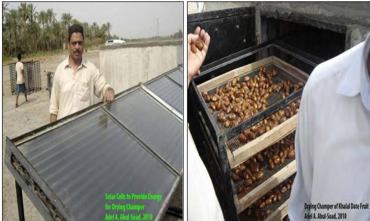
Figure 12: Dates Dehydrators Installed by Pakistan Agriculture Research Council (PARC) project at Khairpur using Solar Energy
