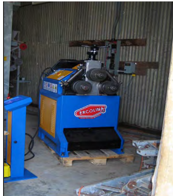
Pipe bender used to manufacture metal ribs in Christiana
