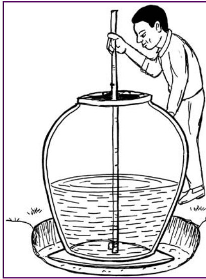
Half-full leak test
