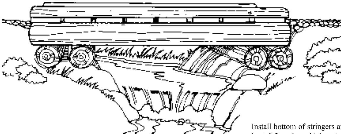
Figure 10.2 Bridge installation with simple foundation details.
