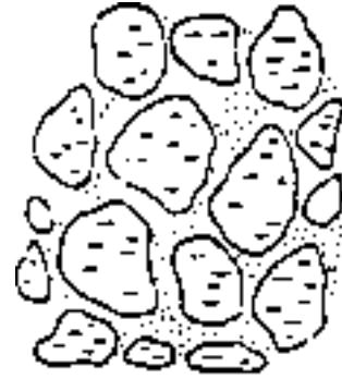
Aggregate with High Amount of Fines (>30 percent)
