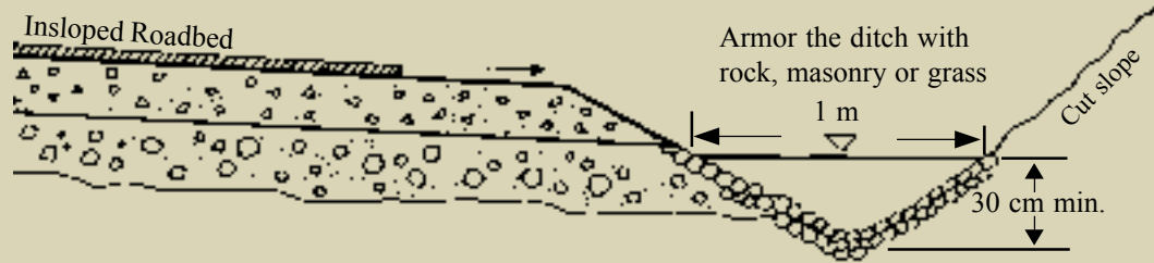
b. Typical Ditch Armoring and Shape
