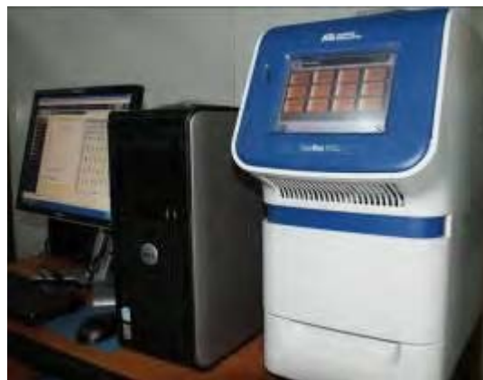
The PCR installed and ready for use
