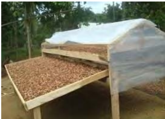
Solar dryer with rack model that allows for double the capacity in Polman
