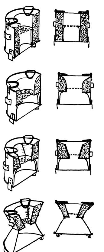
The traditional metal stove lined with insulation all the way down. Proved to be too bulky and weighty.
