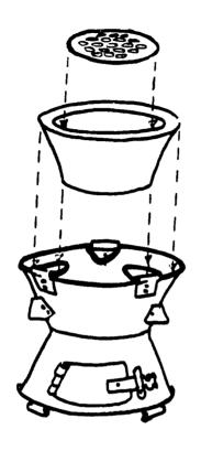
(f) The Kenya Ceramic Jiko. The ceramic liner was altered to line only the top half of the stove. This reduced the weight of the stove considerably, simplified construction technique (thus reducing construction costs), and provided more space in the ash chamber which also improved the ignition time.
