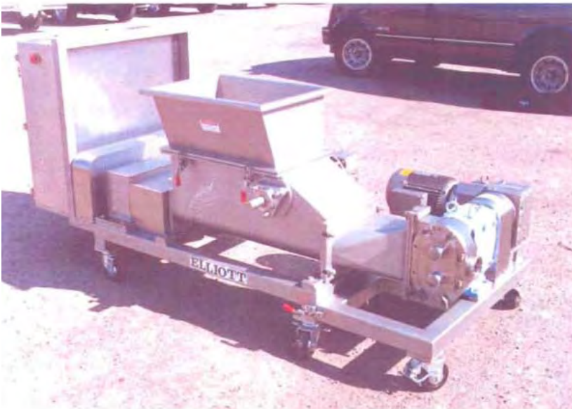
← Date Paste Pumping System
