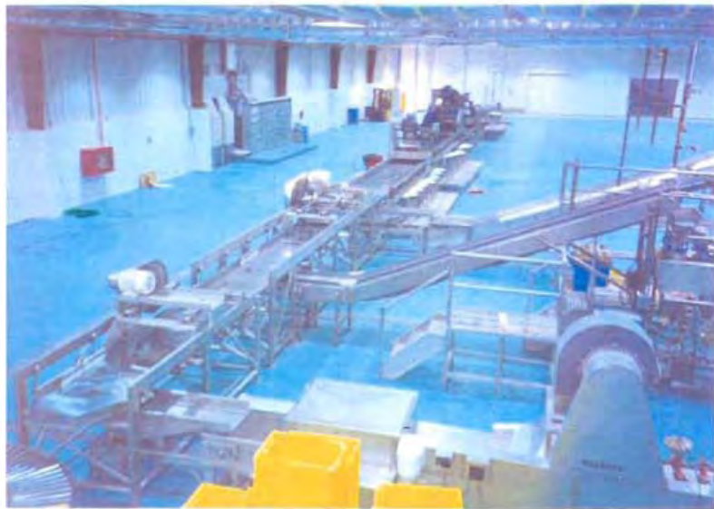
▲ Distribution Conveying to Paste and Press Equipment
