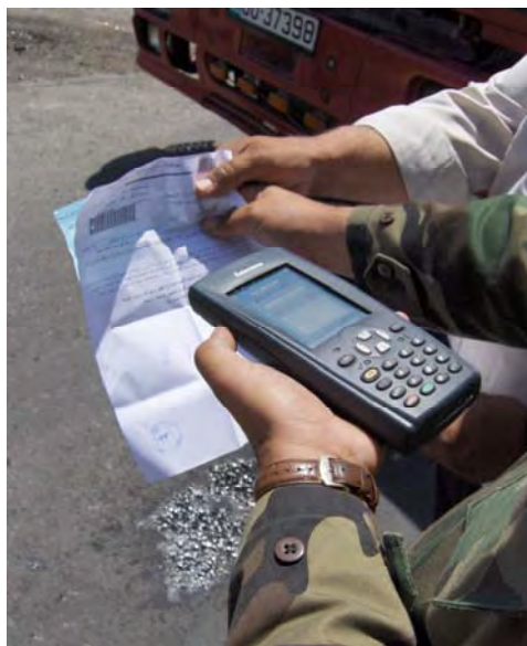
A Jordan Customs officer utilizes a handheld computer and barcode scanner as part of the gate control system.
