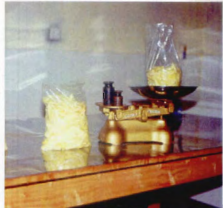
Plates 9-12. Par-fried samples of French fries are weighed (top), packaged and deep frozen (bottom) for subsequent use in fry colour determination and sensory tests
