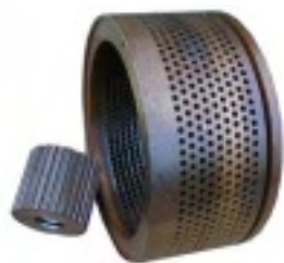
Figure 8.2 Key parts for pellet production (roller and die)
