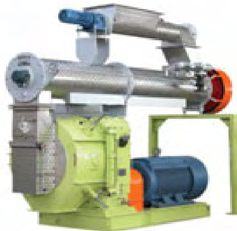
Figure 8.3 Example of a small pellet machine with a capacity of 300 kg/hour.
