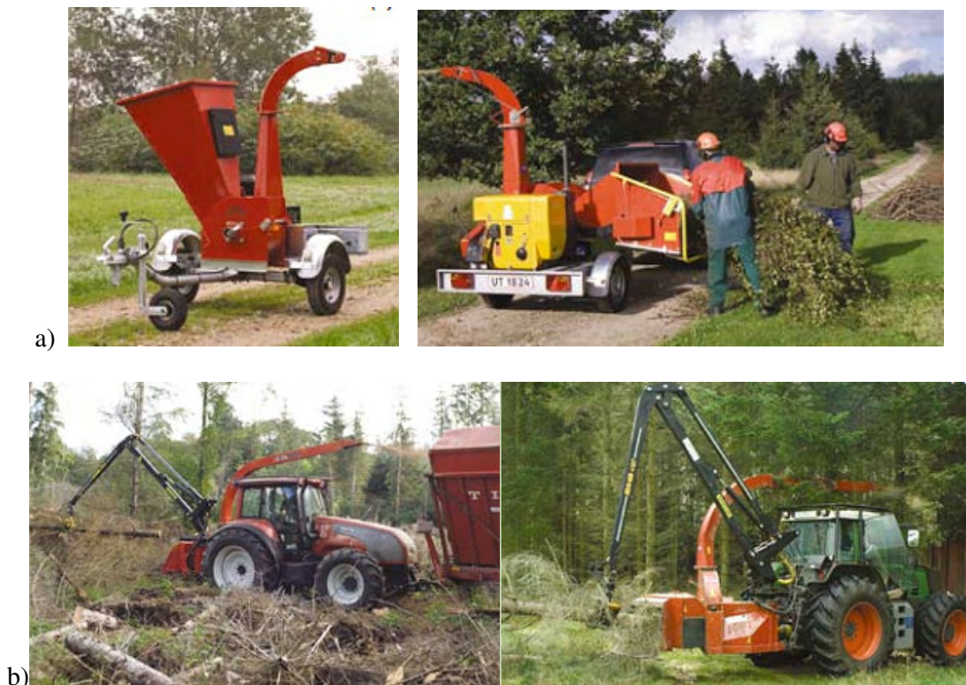
Figure 6.1 Machines for woodchip production ( www.linddana.dk )
