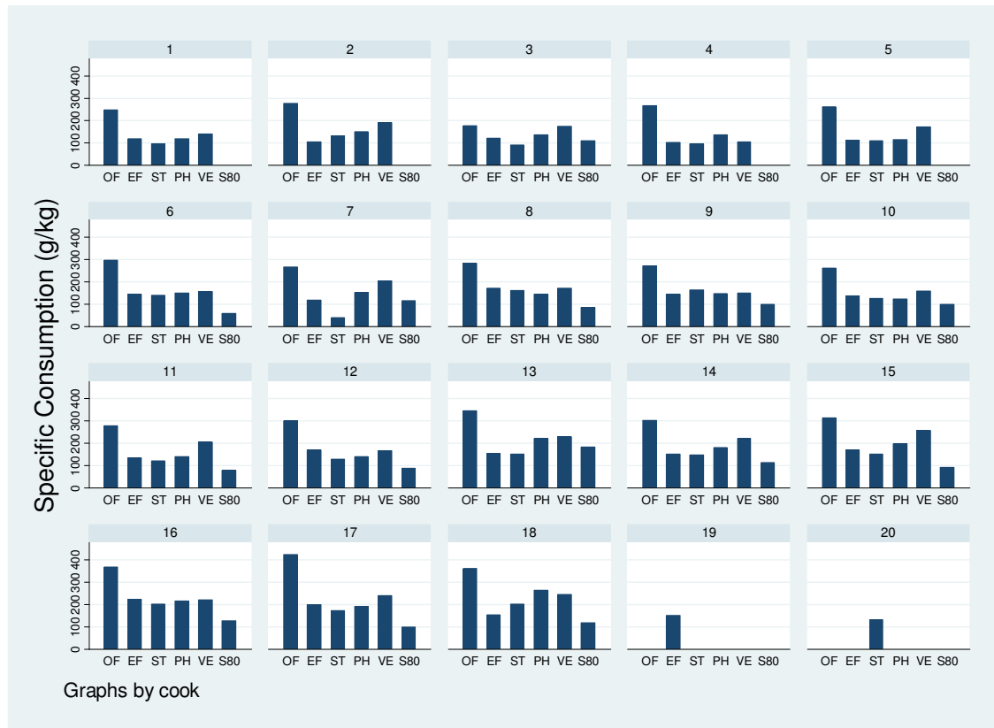
Figure A1. Average specific consumption (g/kg) for each stove type for each of the cooks.
