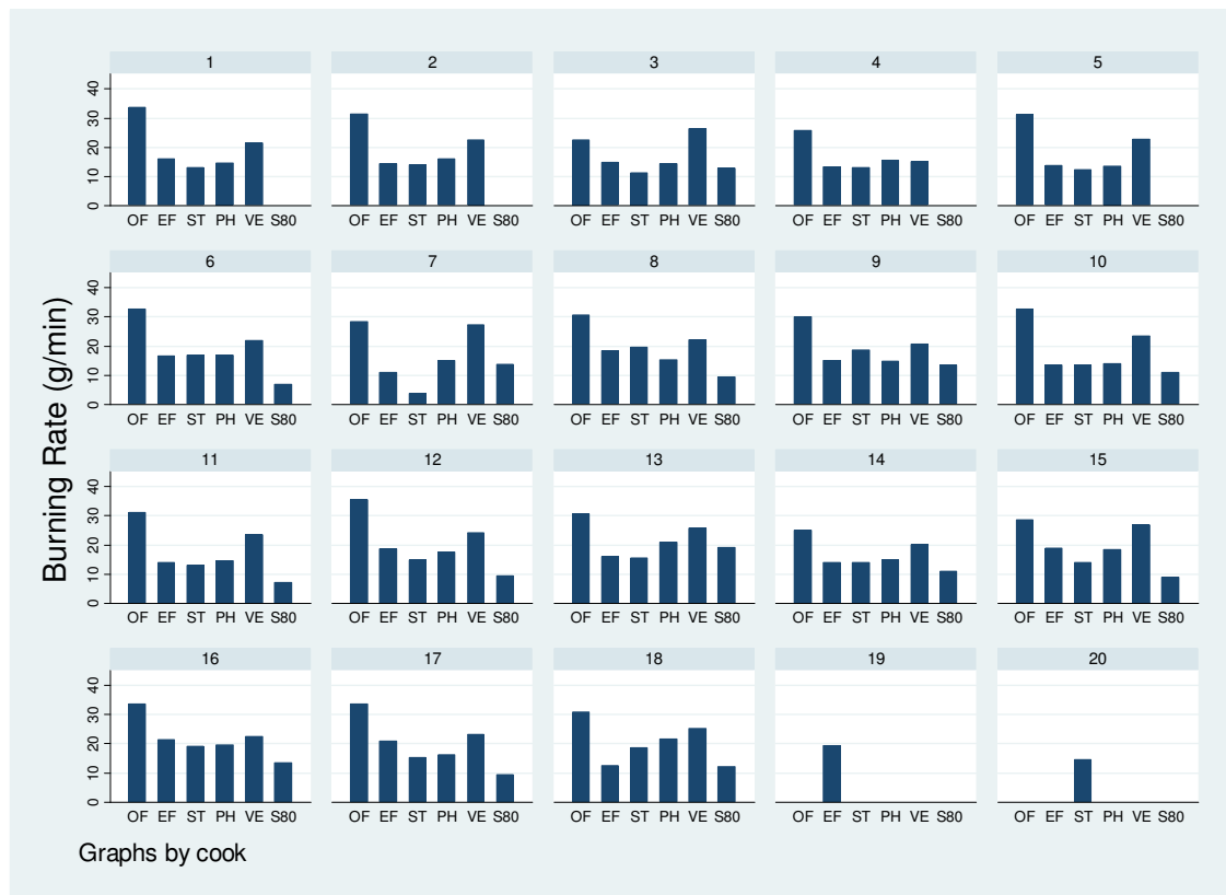
Figure A3. Average burning rate (g wood used per minute) for each stove type for each of the cooks.
