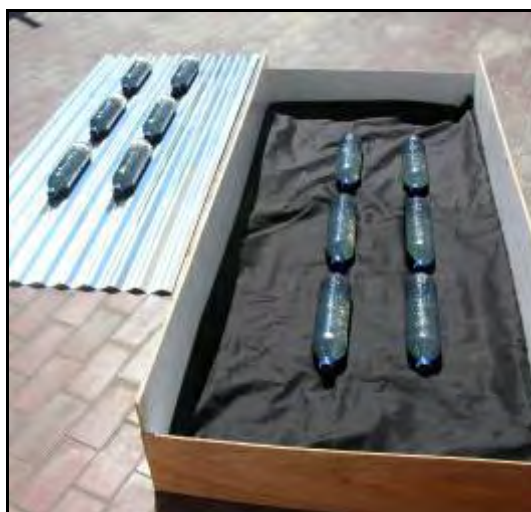
Figure 4-3 SODIS Bench-Scale Experiment in Jakarta
