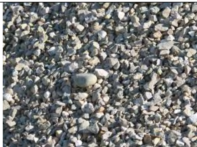
Aggregates with different origin (not clean)
