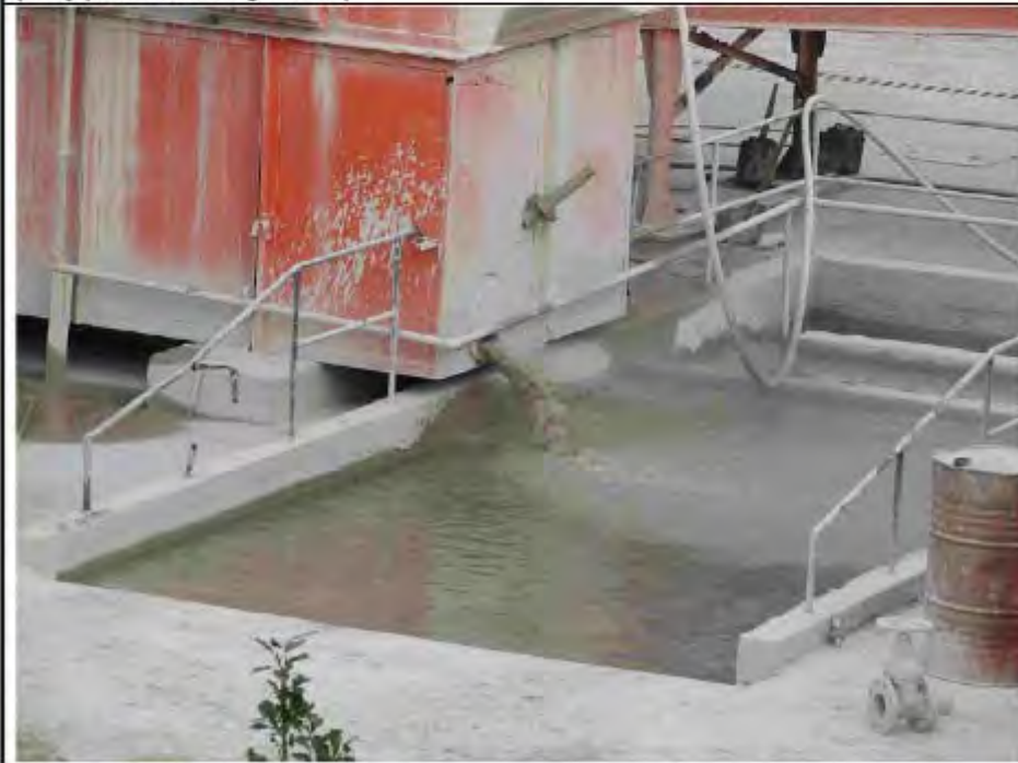
Dust (filler) filter system
