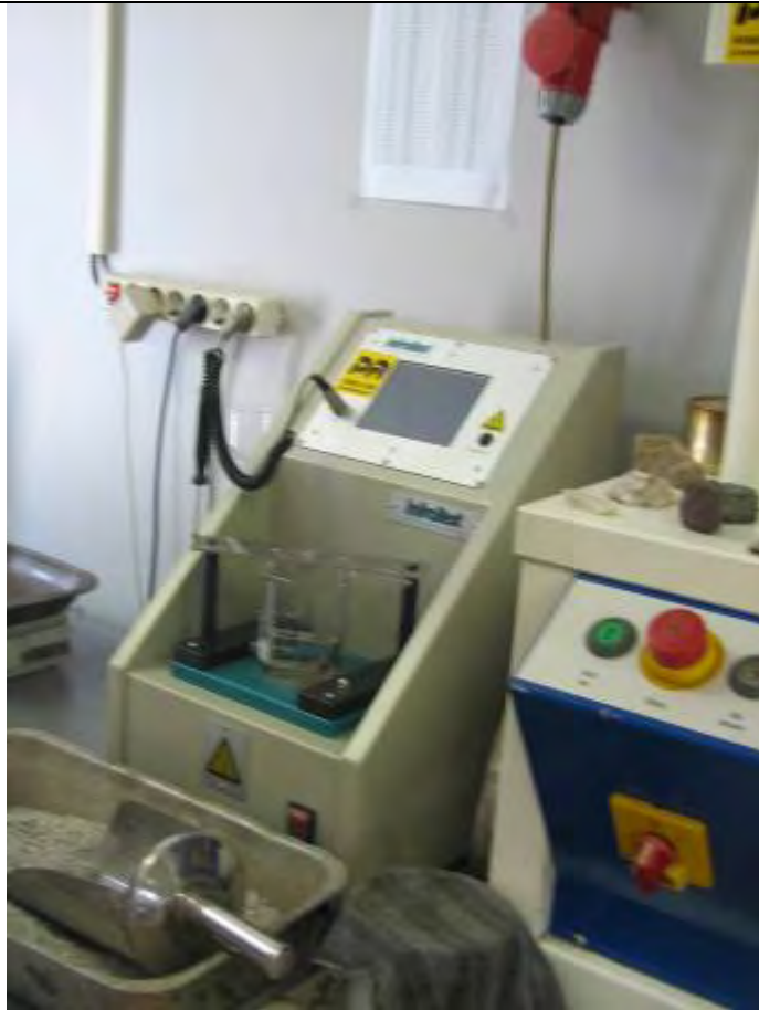
Ring and ball bitumen test device (automatic)
