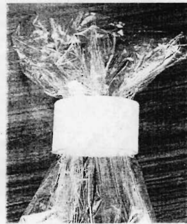
Figure 2. Plastic 'collar' for closure of plastic culture bags.
