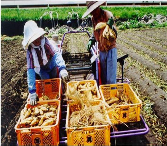
Figure 4. One-row chain type digger capable of harvesting 1 to 1.5 hectares per day.
