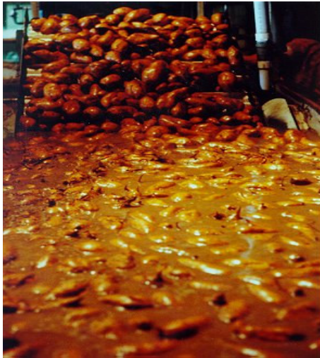
Figure 25, left. Dumping roots in a tank of water will remove most of the surface dirt.
