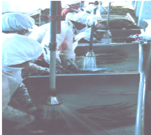
Figure 4. Overhead spray wash cleaning of green onions in a large-scale operation.
