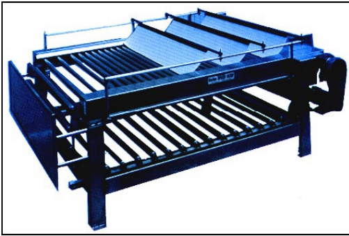
Figure 7. Rotating bar-sizer for categorizing tomato fruit.
