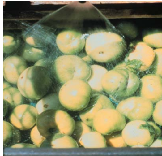
Figure 5. Over-head spray of high pressure water for cleaning mature green tomato fruit.
