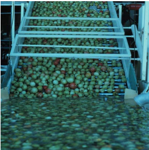
Figure 4. A properly sanitized wash tank is essential to minimize postharvest decay.
