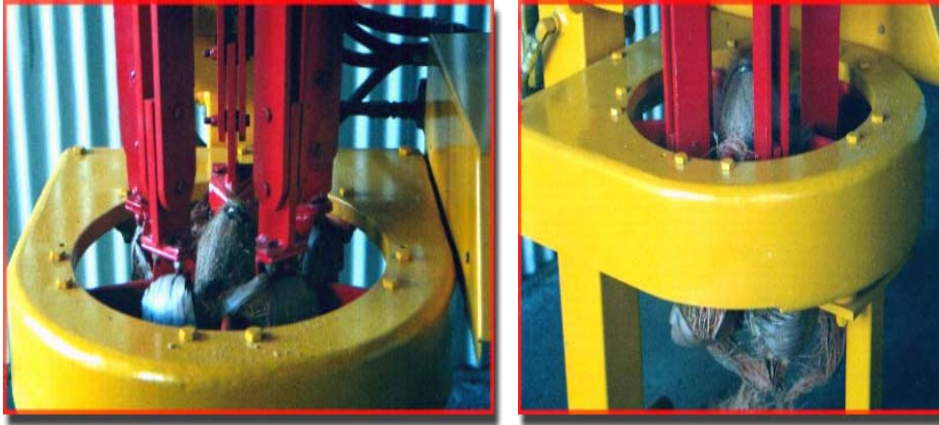
Figure 8. The husking arm assembly splits open the husk (left) and removes it from the coconut (right).
