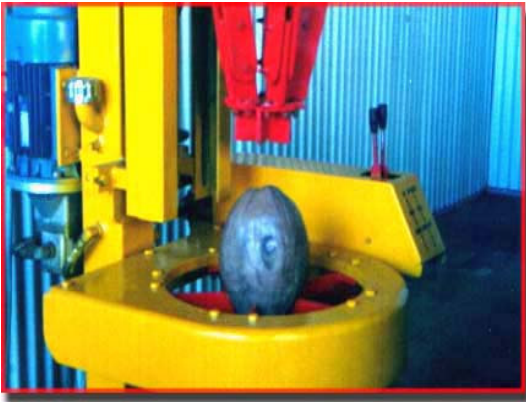
Figure 6. Coconut resting on the base knives with the fruit attachment scar pointing to the center of the husking arms.
