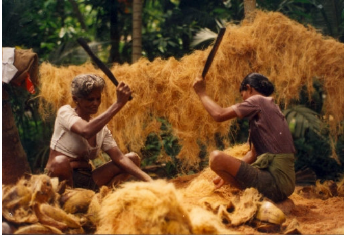
Figure 12. Manual pounding of coconut husks with wooden mallets against stone or slabs of wood to extract the fiber.
