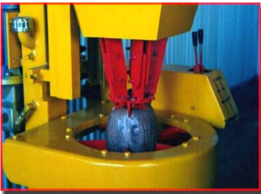
Figure 7. The husking arm assembly is lowered until good penetration into husk is attained.
