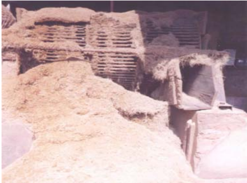
Figure 14. Mechanical separation of coconut husk fibers using a series of rotating chains.
