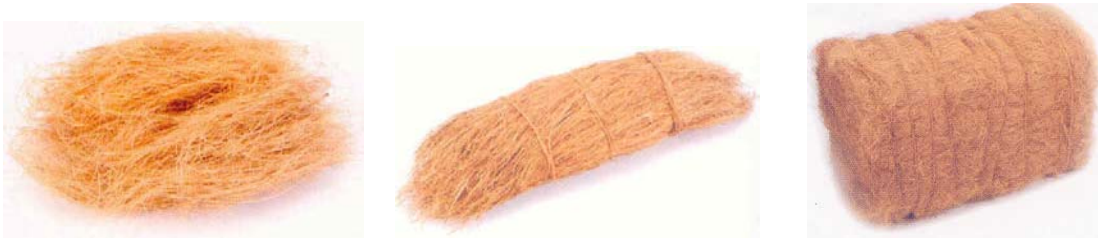
Figure 19. Various types of coir fiber include: mattress fiber (left), bristle fiber (center), and un-retted fiber (right).
