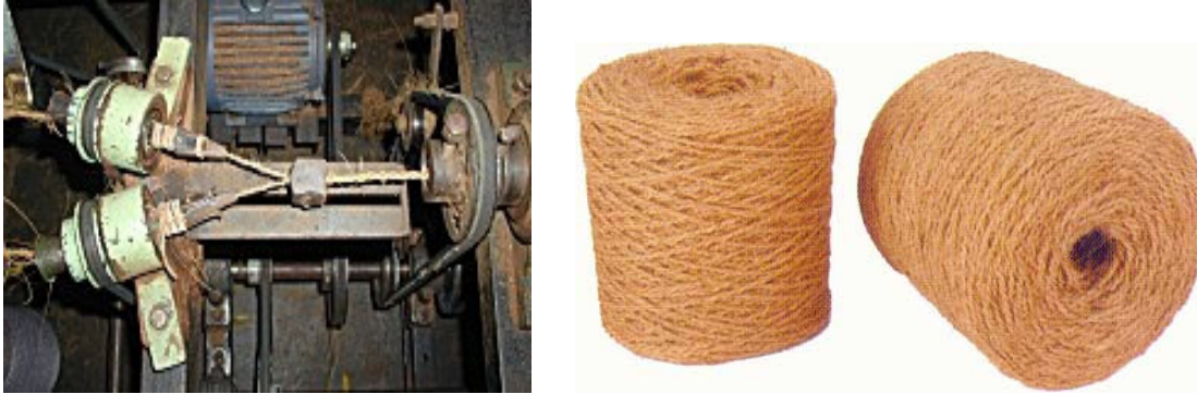
Figure 21. Machine (left) for spinning coir fibers into bobbins of yarn (right).
