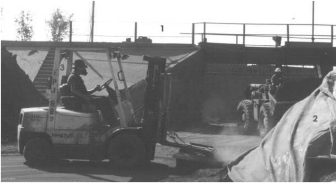
Figure 6. Storage area in May 2000, showing higher fences (1), covered and moistened ore piles (2), and workers in filter masks (3). Courtesy of Carlos Sanchez
