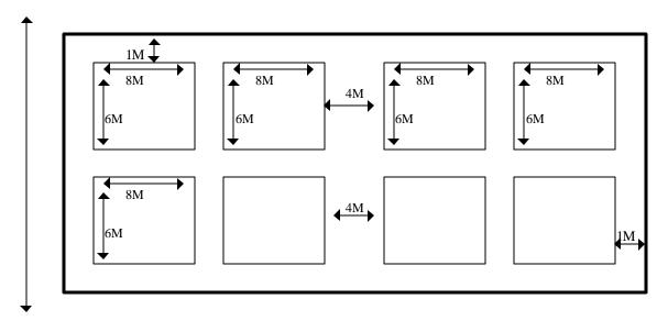
Gross volume =  $40M \ge 15M = 600M^2 \ge 5M = 3,000M^3$ Usable volume =  $(40M - 4M - 4M) \ge (15M - 3M)$ =  $32M \ge 12M = 442M^2 \ge 4M = 1,768M^3$ Storage Capacity =  $1,768M^3 / 2 = 884M^3$  (17,680 bags) (Source: CARE Food Resource Manual, November 1995).
