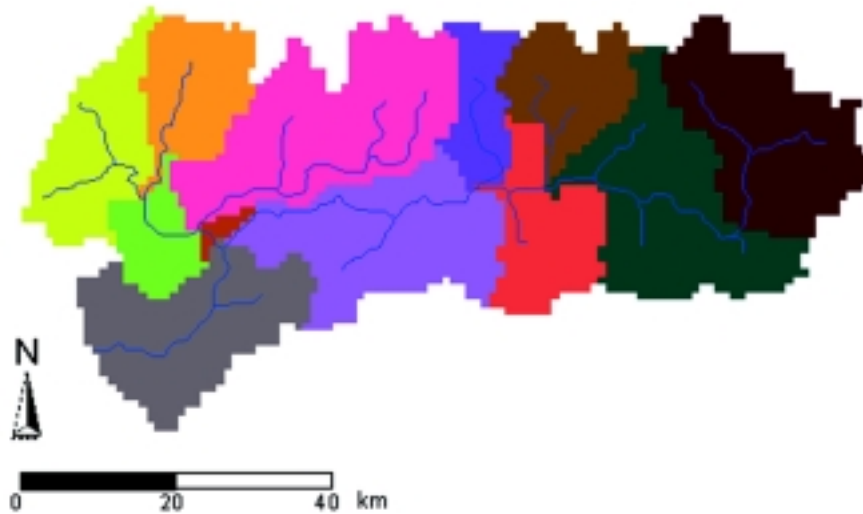
FIGURE 3. Subbasins determined from topographic analysis of the USGS DEM.
