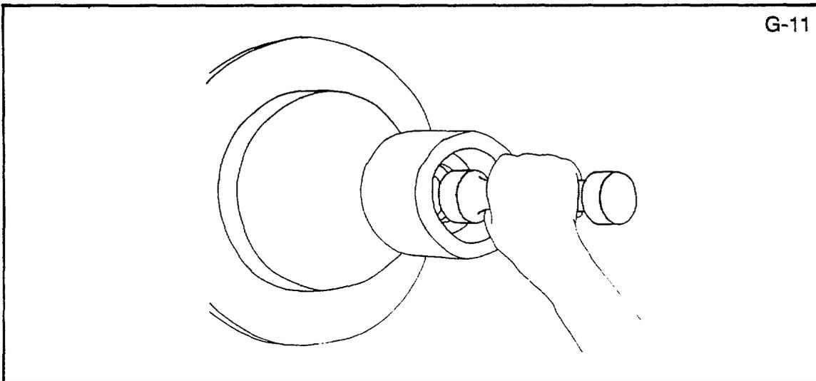
**Inspection 5b.** "Go" part width gage must fit into seating surface; "no go" part must not fit into seating surface.
