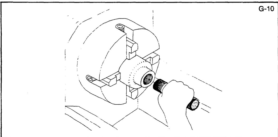
**Operation 4.** Bore seating surface for valve seat (lower cylinder end only).
