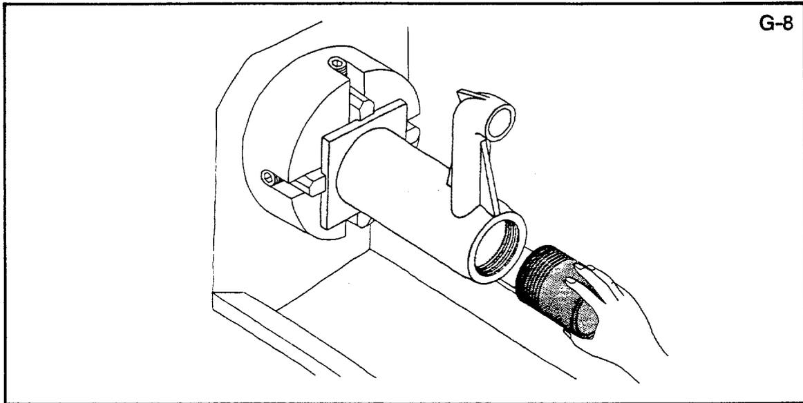
**Operation 3.** Drill four holes using fixture.
