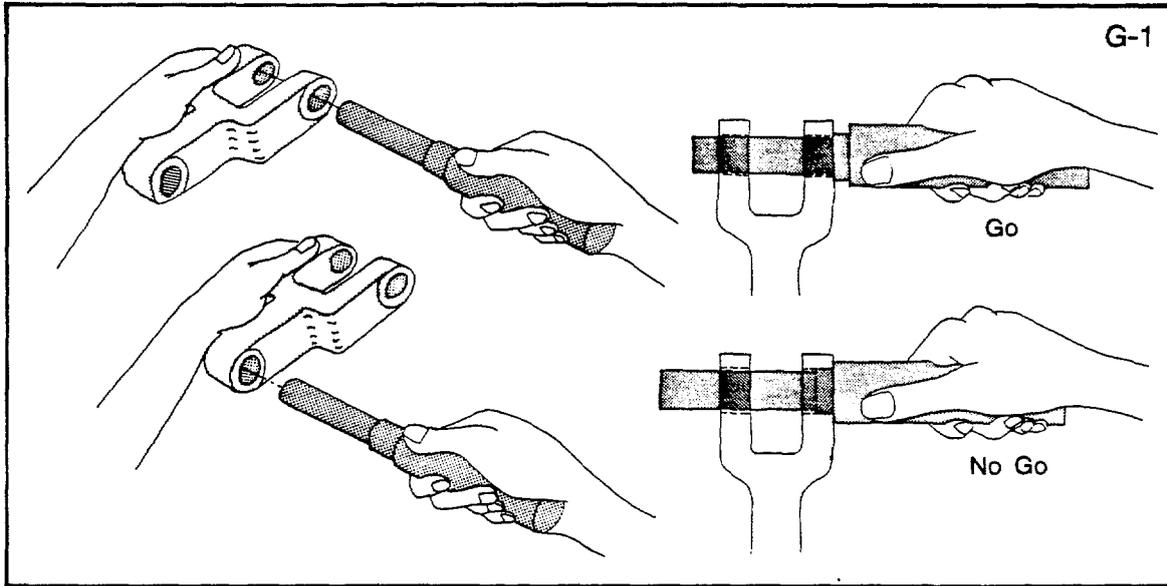
**Inspection 2b.** Measure distance between holes; gage must fit through holes.
