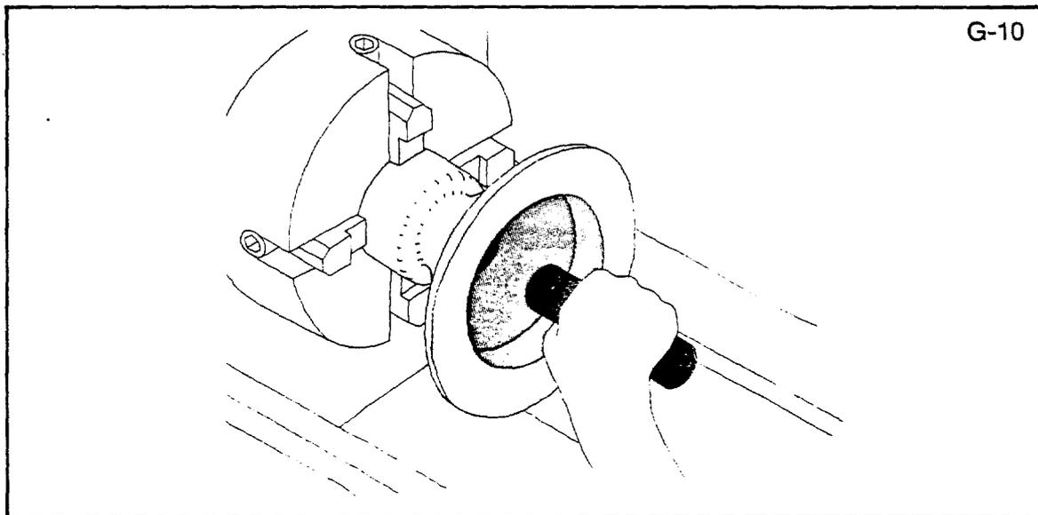
**Operation 3.** Cut pipe threads in upper pump base.
