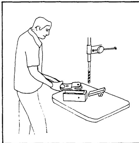
**Inspection 2a.** Measure reamed hole diameter with gage; smaller diameter of gage must fit hole but larger diameter must not.
