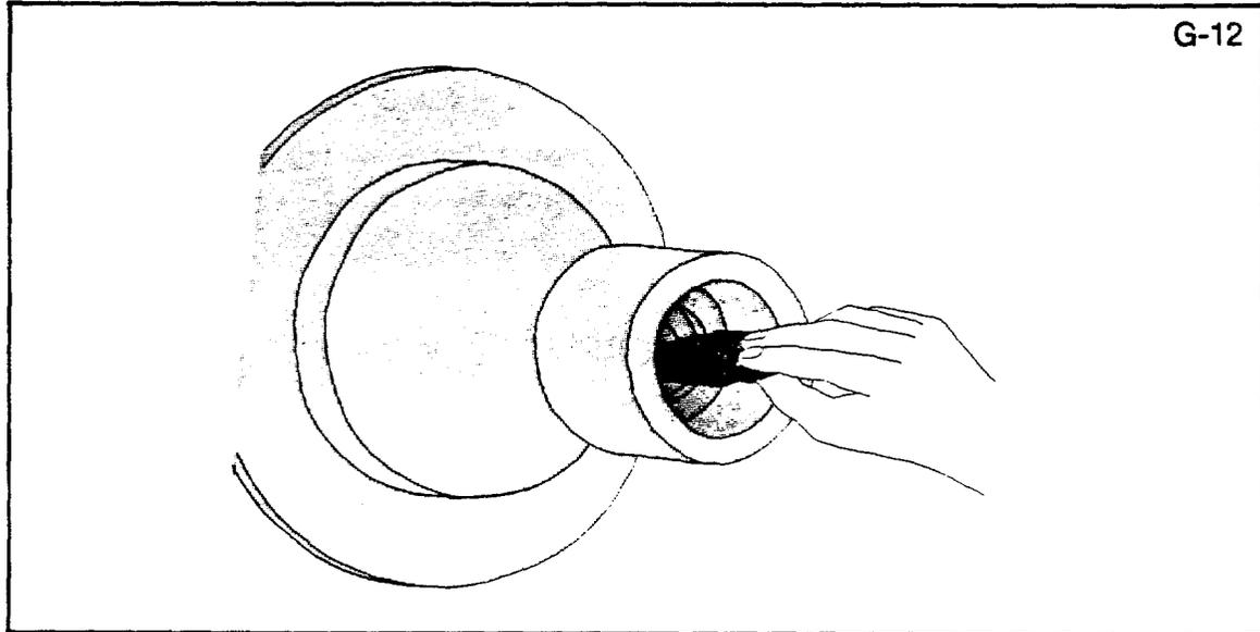
**Inspection 5d.** "Go" part of depth gage must not touch seating surface; "no go" part of depth gage must touch seating surface.
