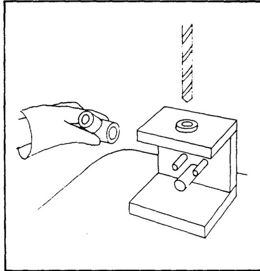
**Inspection 3.** Tapped hole must fit gage.
