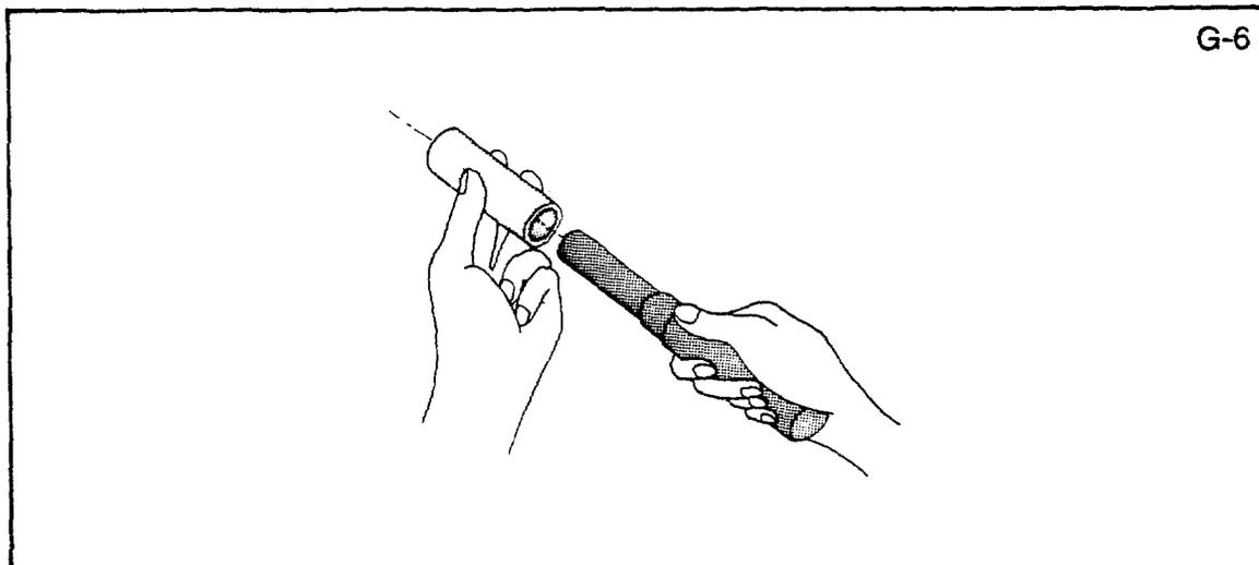
**Operation 3.** Cut off and chamfer bushings.
