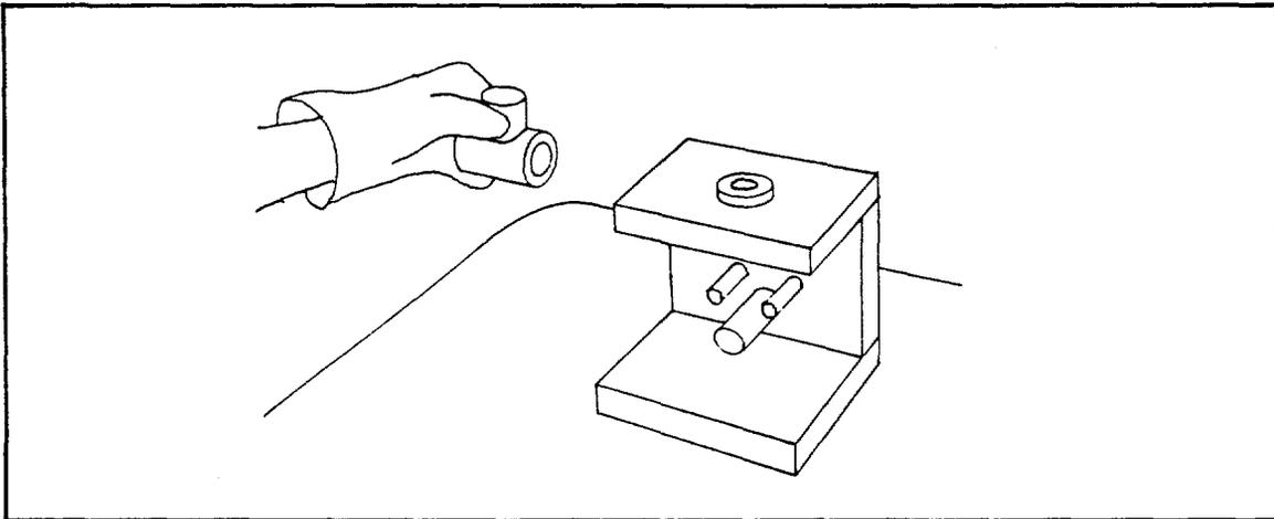
**Operation 3b.** Drill hole for plunger rod; thread hole.
