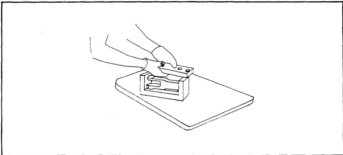
**Operation 2b.** Drill two holes in fulcrum; ream both holes.
