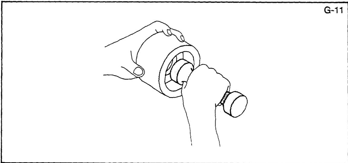
**Inspection 4b.** "Go" part of width gage must fit into seating surface; "no go" part must not fit into seating surface.
