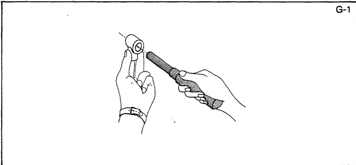
**Operation 3.** Drill and tap hole for plunger rod.
