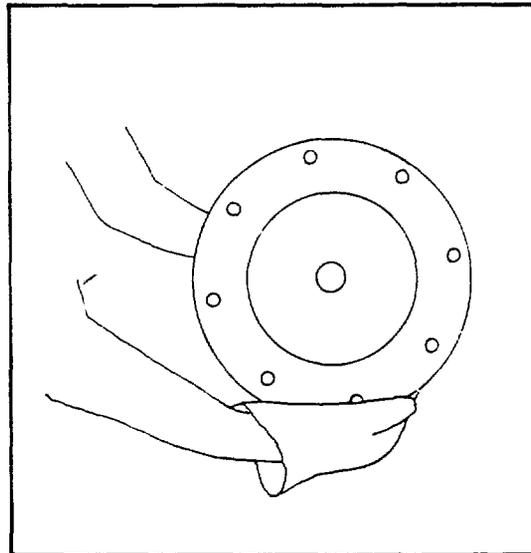
**Operation 5.** Bore seating surface for valve seat (shallow well pumps only).
