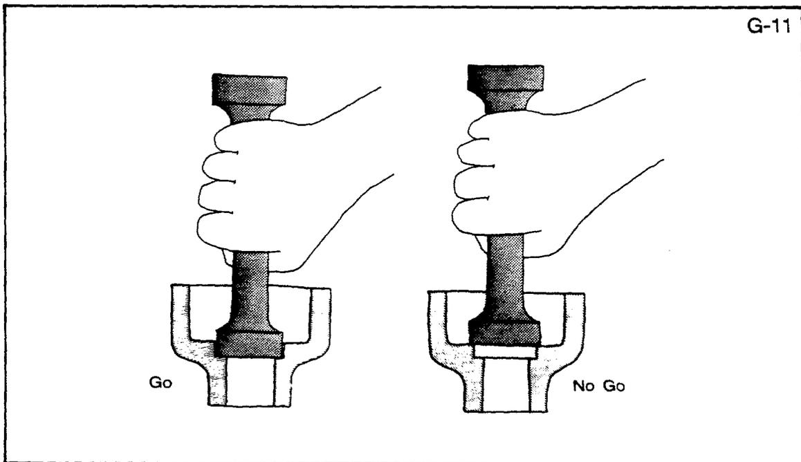
**Inspection 4c. Measure depth of seating surface**
