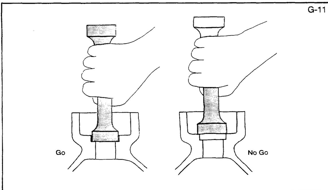
**Inspection 5c.** Measure depth of seating surface.
