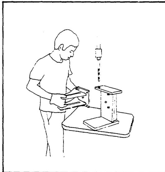
**Inspection 4.** Measure reamed holes; small end of gage must fit holes,
