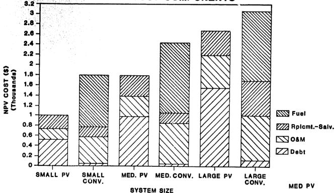
For this evaluation, PV- and diesel-powered multi-use systems are compared, assuming development agency financing. Exhibit E-20 provides the base-case parameters used in this comparison. Multi-use systems are the least-cost option for average energy demands less than 2 kWh/day. Between 2 kWh/day and 16 kWh/day, PV system financial viability is in the break-even range, dependent on case-specific parameters. Above 16 kWh/day, PV multi-use systems are not currently financially viable.
