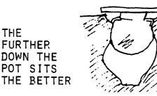
Arrange for the pot used to cook foods requiring highest - heat to be over the firebox hole. In Guatemala, this is where the skillet, or comal, used in making tortillas fits.
