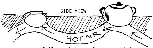
Build-up bottom of each pot hole leaving a three finger space.
