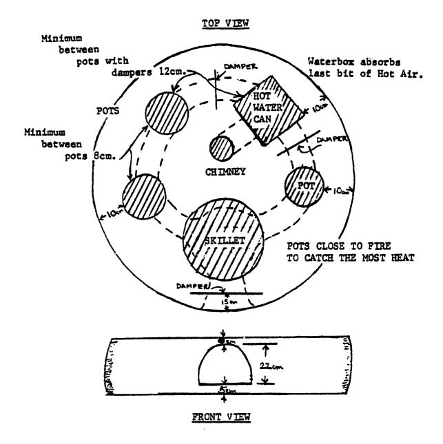
Locate the firebox at the fron center of the stove. Arrange pots so that they are closest to the heat source. Diagrams show the positions of hot air tunnels and dampers; a cooking hole located near the chimney provides enough heat to keep water warm for washing.
