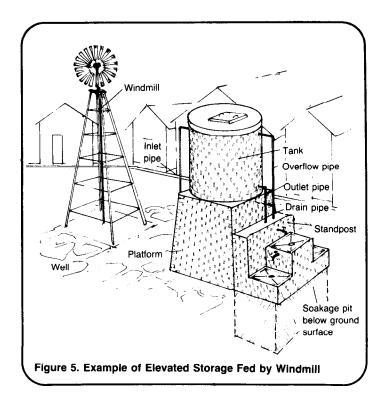
Storage tanks can be made of rock masonry or ferrocement. Ferrocement requires the use of bricks and wire mesh reinforcement. A weld mesh frame and chicken wire to form and support the walls are used.
