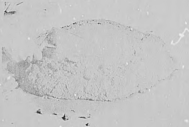
Fig. 9. This mix is too sandy because it contains too much sand and not enough coarse aggregate. It would place and finish easily, but would not be economical, and would be very likely to crack.
