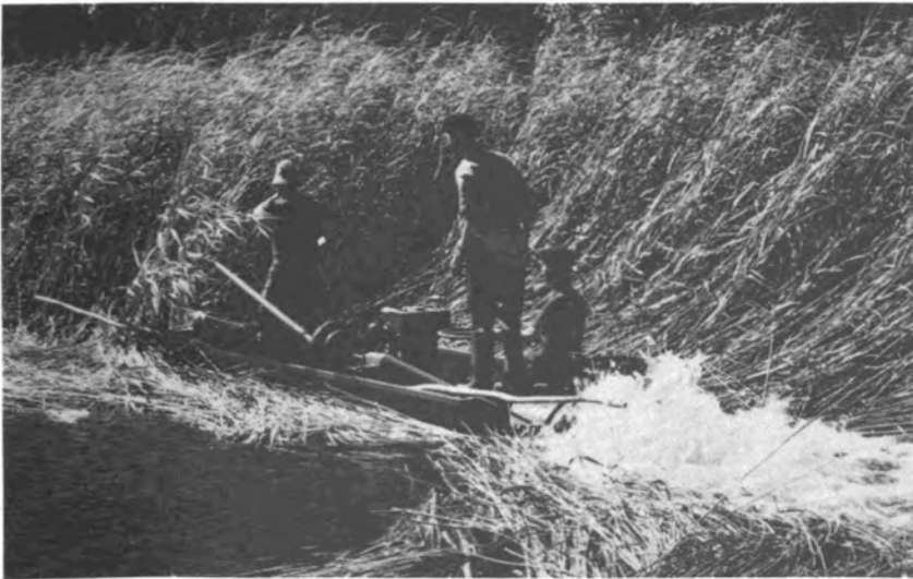
A small mowing boat, particularly suited to cutting reeds and other emergent aquatic weeds. (Krinke and Krüger G.m.b.H., Langenhagen, Federal Republic of Germany)
