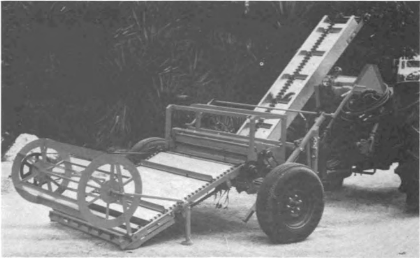
Tractor-powered, mobile harvester for water hyacinth or other floating aquatic weeds. (L. O. Bagnall)
