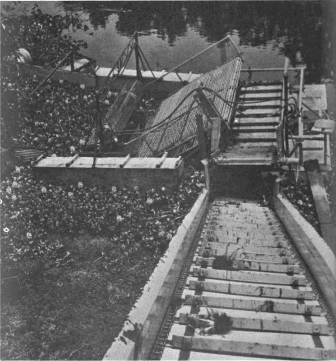
Conveyors with feeders require little energy to remove aquatic plants from the water and lift them to processing or transportation equipment. They can be made in a wide range of sizes and complexities. This one is on the St. John's River, Florida, USA. (Aquamarine Corporation)
