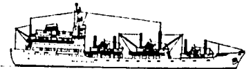
Vessel type: Mother Ship Number in crew: 183 Length overall: 377'. Six catcher boats are carried on deck. Also serves as factory ship.
