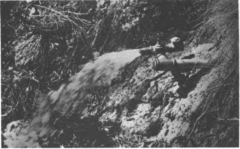
FIGURE 37 A completed horizontal well on test yields over 50 gpm. Plumbing head includes two tees, a shutoff valve to regulate the flow, a vacuum relief, and a pipe reducer. (W. T. Welchert)
