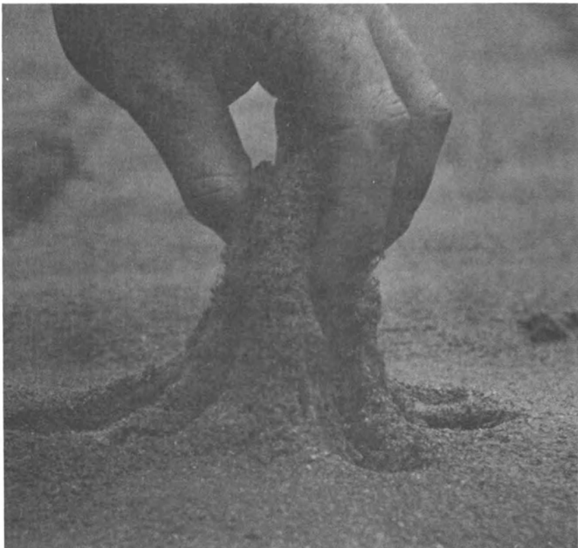
FIGURE 54 Consistency of sand stabilized with an oil/latex mulch. Sealed surface reduces evaporation losses and holds the sand in place long enough for plants to become established. (International Synthetic Rubber Company, Ltd.)
