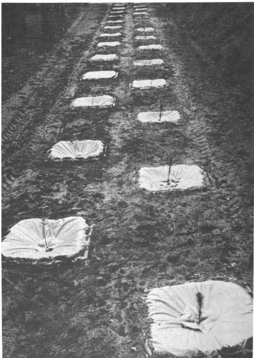
FIGURE 52 These plastic "aprons" are being evaluated to determine their ability to catch rainfall (chapter 2), reduce evaporation, suppress weeds, and promote the growth of tree seedlings in arid areas. (FAO)
