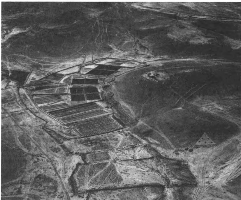
FIGURE 15 Reconstructed ancient farm at Avdat in the Negev. Farm is, and was, watered by runoff from surrounding slopes and wadis. In the foreground are four reconstructed terraces; in the background, four reconstructed channels lead runoff to the farm. To the right are traces of three channels that once carried runoff water to the lower terraces. Ratio of catchment to cultivated area is 20:1—each ha of cultivated land receives runoff from 20 ha of slopes, as well as direct rainfall. Cultivated area receives water roughly equal to a rainfall of 300-500 mm from actual rainfall of 100 mm. (L. Evenari)
