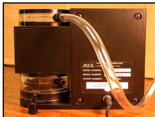
Figure 3: Tube to cyclone connects to upper outlet of calibrator.
